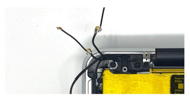
c. Cut 1cm lengths of **BLACK** heat shrink and slide these onto the remaining antenna cables.
