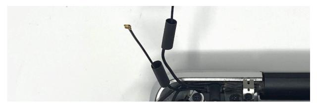
d. Carefully slide the heat shrink over the connectors and shrink them either using a hot air gun or hair dryer.
